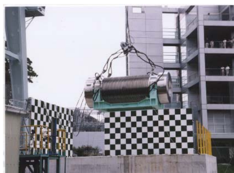
Figure 1. Test of NFT-32B Package Specimen Simulating a Drop Accident at a Loading Wharf of a Ship Port
