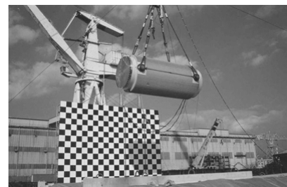
(c) Horizontal drop test from 5 m height
