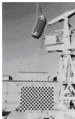
(b) Oblique drop test from 17 m height
