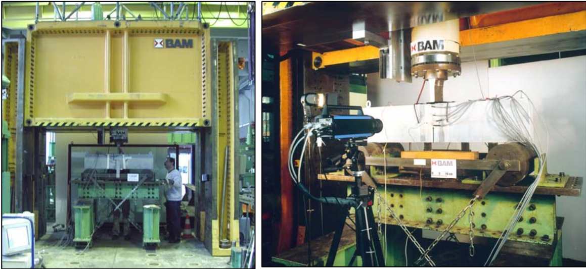
Figure 3. Servo-hydraulic impact test system mounted for dynamic fracture toughness tests with SE(B)140 specimens
