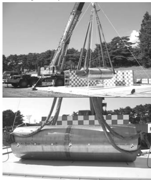
Figure 15. Overall view of the horizontal drop test
