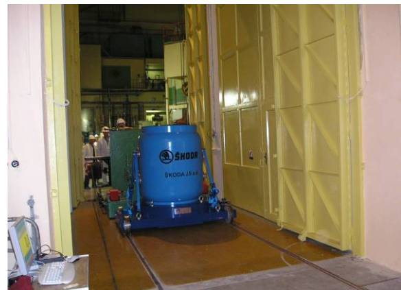
Figure 8. VPVR/M cask being moved into the spent nuclear fuel storage area.
