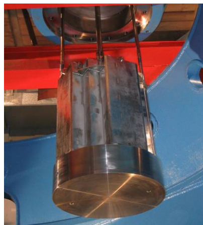
Figure 3. Basket and lower lid being lowered using basket central suspension/hanger and the centering fixture pull rods.
