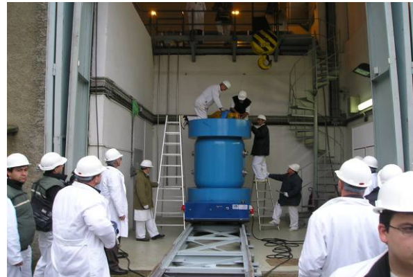
Figure 9. VPVR/M cask being prepared for lifting inside the high-level waste storage building.
