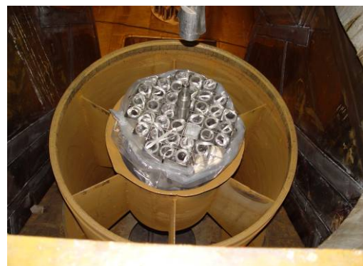
Figure 11. VPVR/M cask basket inside the specially modified Mayak storage pool fuel-handling cart.
