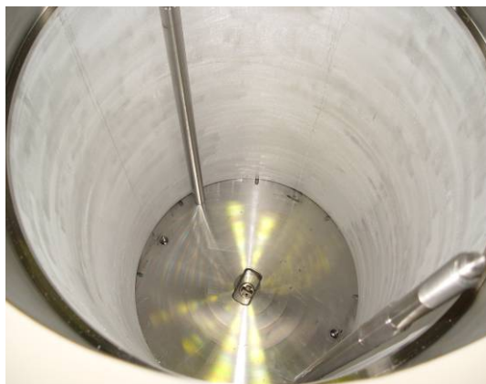
Figure 2. Lower lid central hole with bayonet lock and side pull rods.
