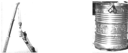
Fig. 4. The 9m free drop test for CDF-1 package designated to liquid wastes (before and after)
