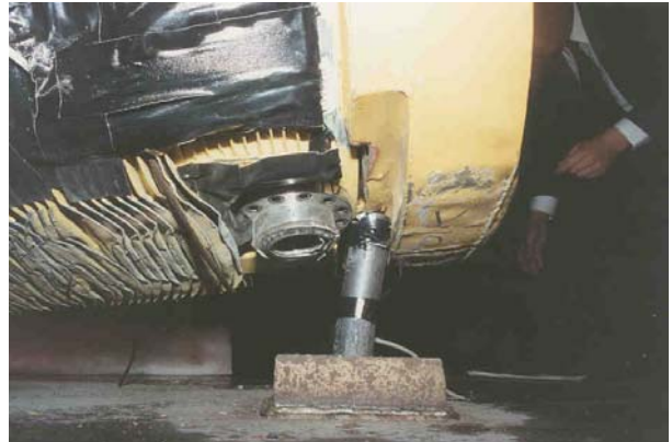
Figure 5. 1/4 Scale side drop and punch test of lid end and shock absorber impact
