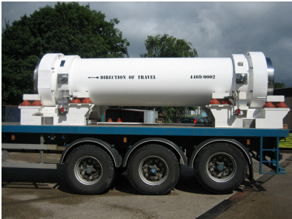
Figure 1: M4/12 MOX package (less shock absorbers)
