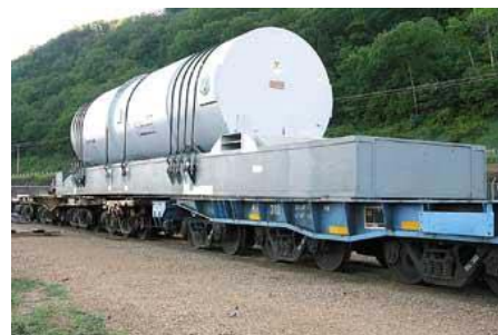
Figure 6 – Rail Transport Configuration
