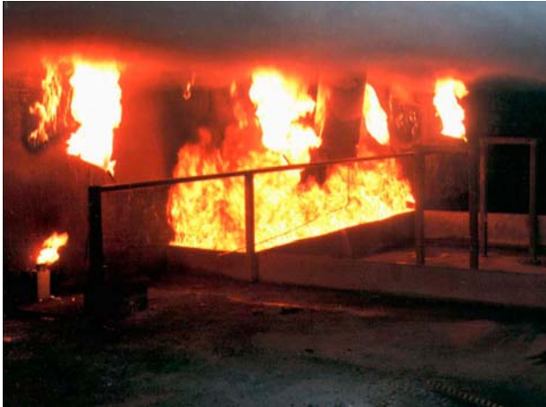
Figure 6 – Heat flux on calorimeter for a 60-minute simulated engine room fire (in addition to the four heptane spray fires there is a pan of burning diesel fuel). The calorimeter was in an adjacent hold on the other side of the bulkhead on the left side of the figure.
