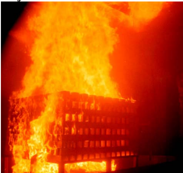
Figure 7 - Heat flux on calorimeter for a simulated cargo fire. The calorimeter was located 1.1 m away from the edge of the wood crib.
