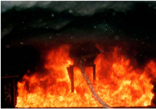
Figure 8 – Heat flux on calorimeter for a pool fire in an adjacent hold. The data shown on the right side of the figure are for a calorimeter in an adjacent hold. The calorimeter seen in the photo was used to provide characterization of the fire.
