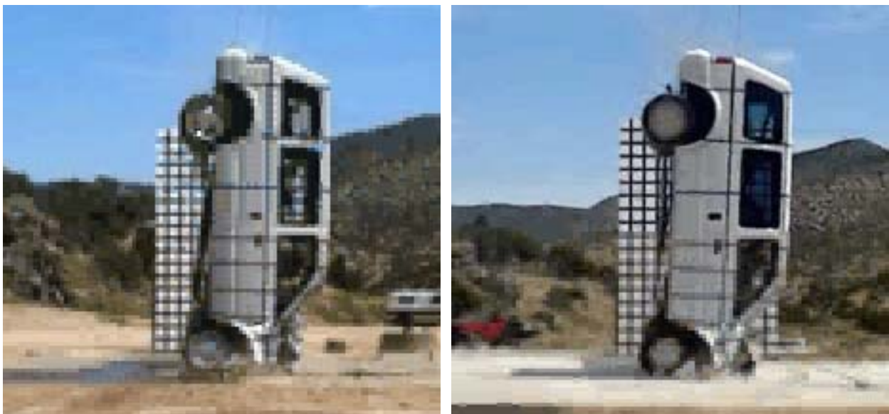
Figure 5 - Comparison of mini-van impact onto an unyielding target (left) and a 28-cm thick concrete slab (right)
