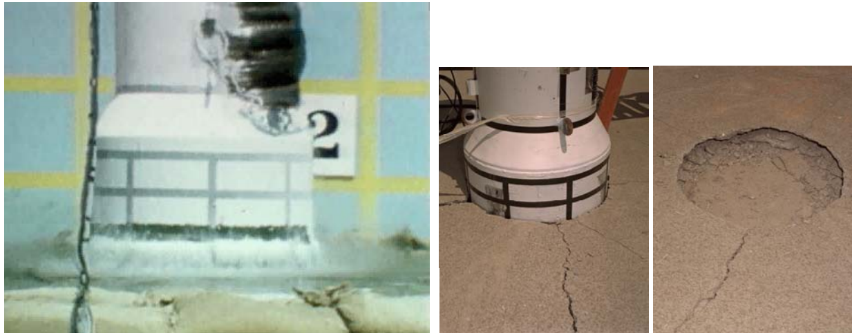
Figure 6 - Comparison of RAM package impact onto an unyielding target (left) and a 28-cm thick concrete slab (right)
