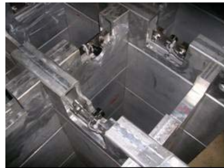
Figure 5. Eddy Current Displacement Sensor inside the Basket
