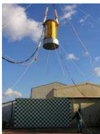
In-house Drop Test with 1/2.35-scale Model
