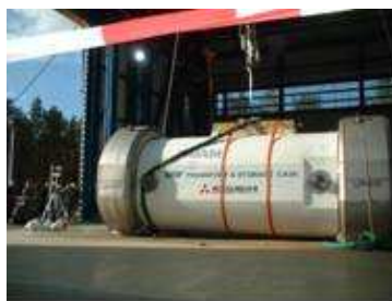
Certification Test with Full-scale Model at BAM Test facility in Horstwalde, Germany
