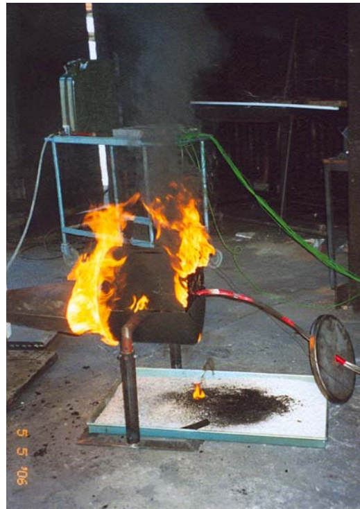
Figure 7: Sample 2 after 21 minutes into the fire test
