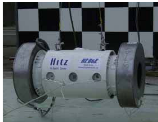
Figure 6. 1/10scale cask model
