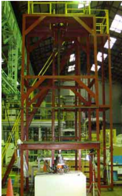
Figure 2. Experimental apparatus of drop weight test
