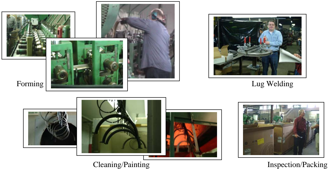
Figure 8 Clamshell Production Process
