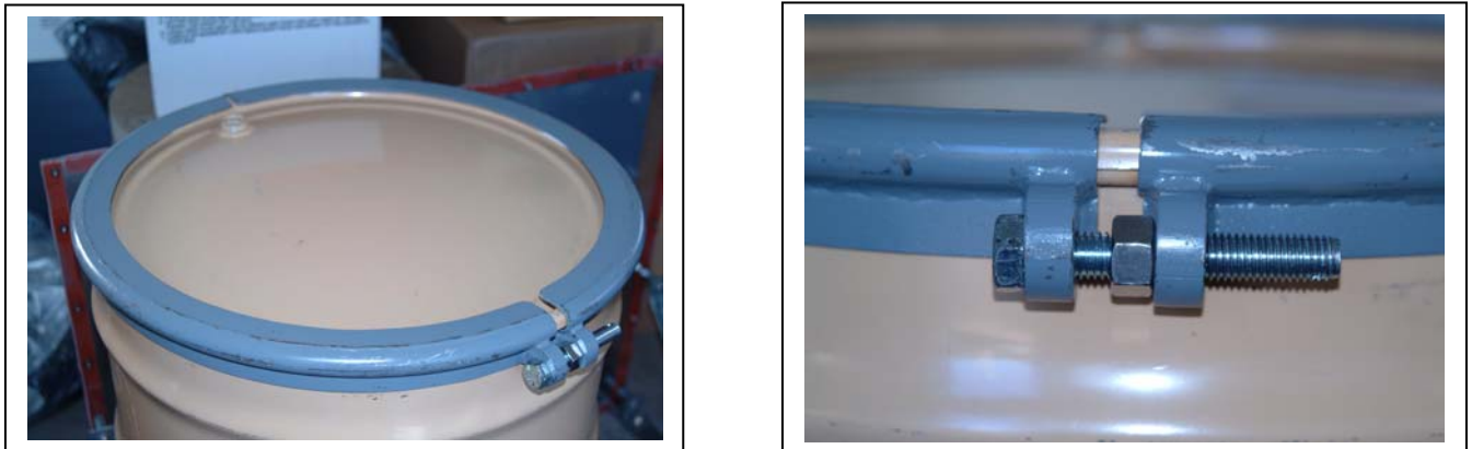
Figure 5 Prototype Clamshell Closure Fitted to a UN1A2 drum
