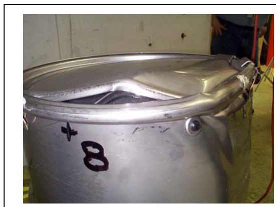
Figure 1 9975 30-ft Drop C-Ring Lid Closure Failure
