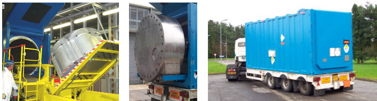
Figure 3. Loading the Transactive (left, middle), TA-20 (right), source: AEA Technology
