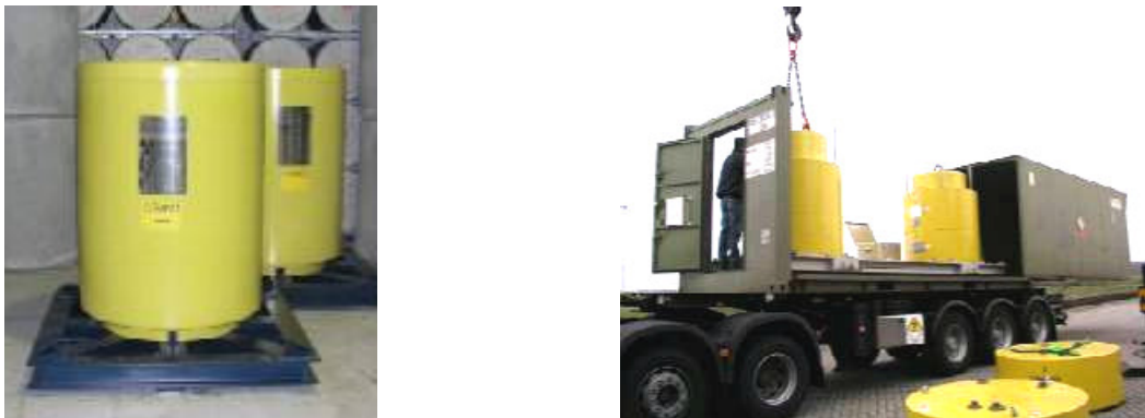
Figure 4. Standard MOSAIK container as interim storage container and in transport configuration with shock absorber in the 20'-Open-All-Container, source: Gesellschaft für Nuklear-Service
