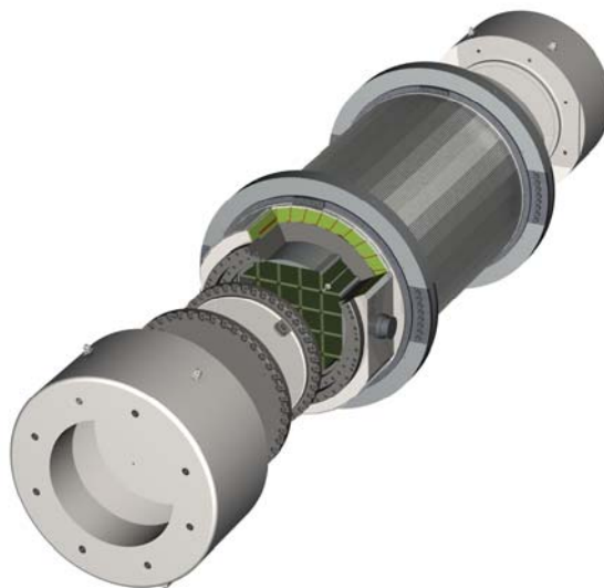
Figure 3: TN 24 E transport and storage cask design
