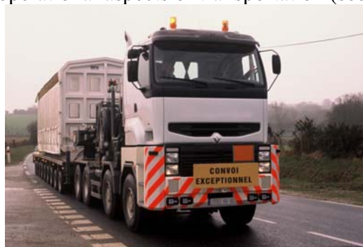
Figure 2: transportation of spent fuel with a LMC (BU-L) truck
