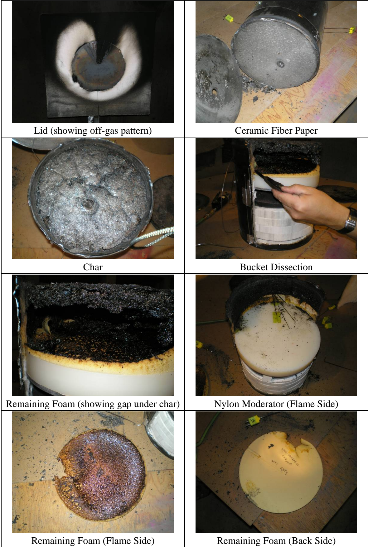
Figure 5 – Post Test Inspection of Bucket 4
