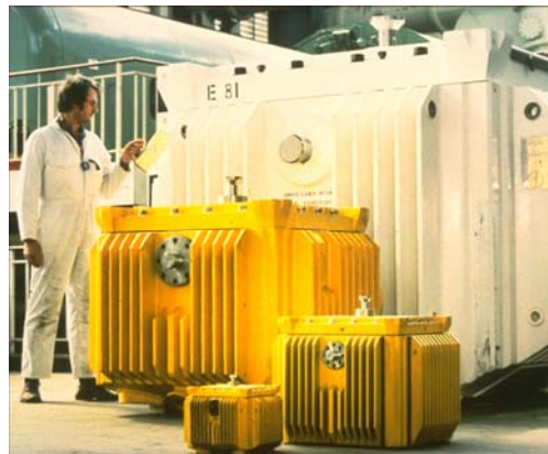
Figure 1. Full scale, and 1/2 , 1/4 and 1/8 scale model, Magnox Fuel Flasks
