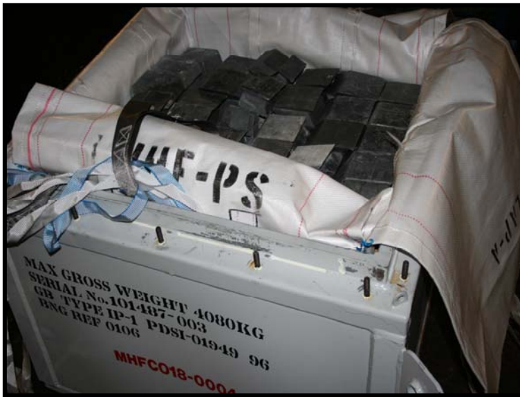
Figure 4 is a photo of the PDSI 01949 package with lift liner installed and filled with radioactive lead chevrons from the Sellafield site in the United Kingdom.
