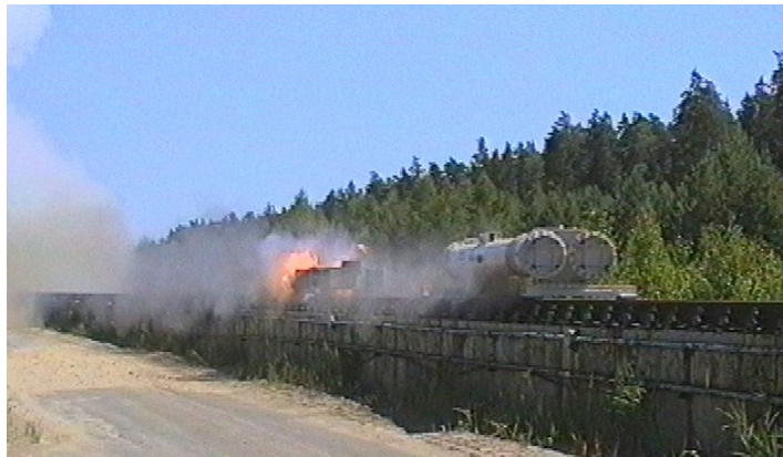
Fig.1 Horizontal rocket track of RFNC-VNIIEF, which is used for tests where casks are impacted against target with velocity not less than 90m/s
