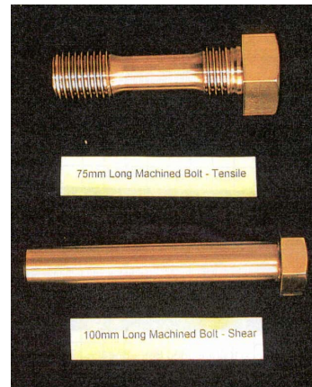
Figure 6: Typical waisted shank bolt for tensile testing and plain bar for shear testing
