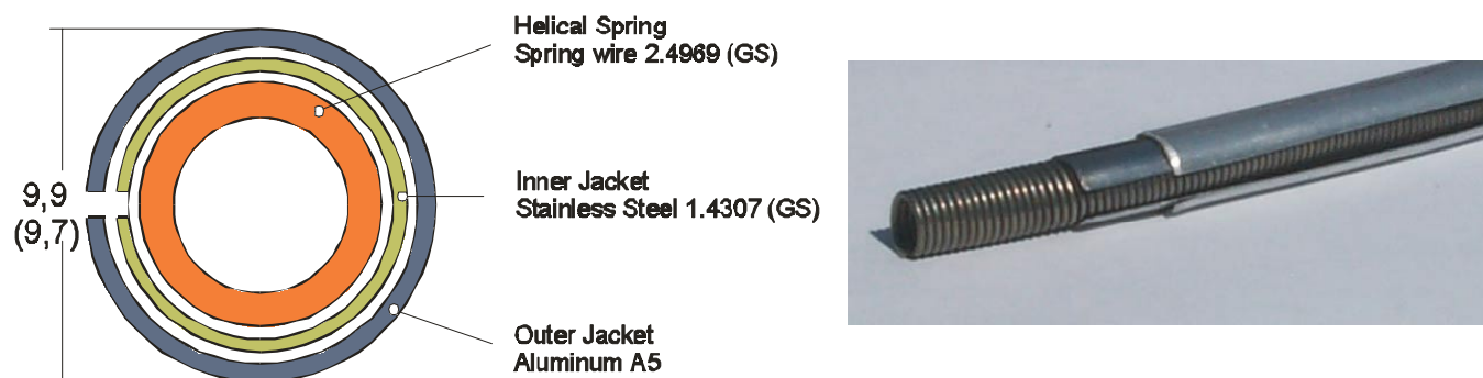
Fig. 1: General structure of "Helicoflex" type metal seals (German nomenclature of material numbers)
