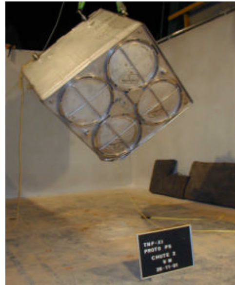
Drop test at COGEMA LOGISTICS' test facility in Laudun (France)
