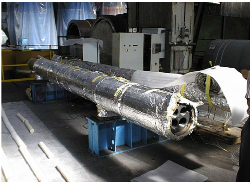
Fig. 6 Cast iron pipe with bore
