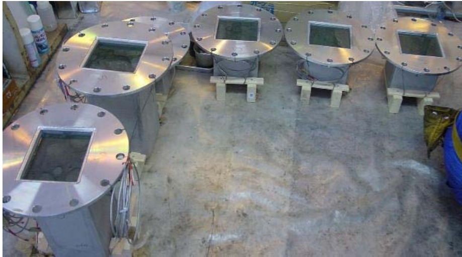
Fig.1 Test Vessels of Neutron Shielding Material (NS-4-FR)
