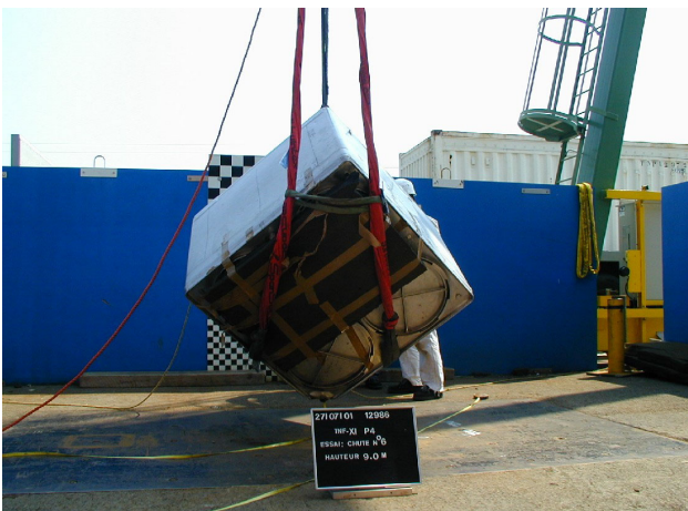
Figure 3 Before 9 m drop test
