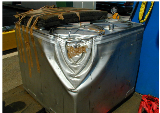
Figure 4 After 9 m drop test
