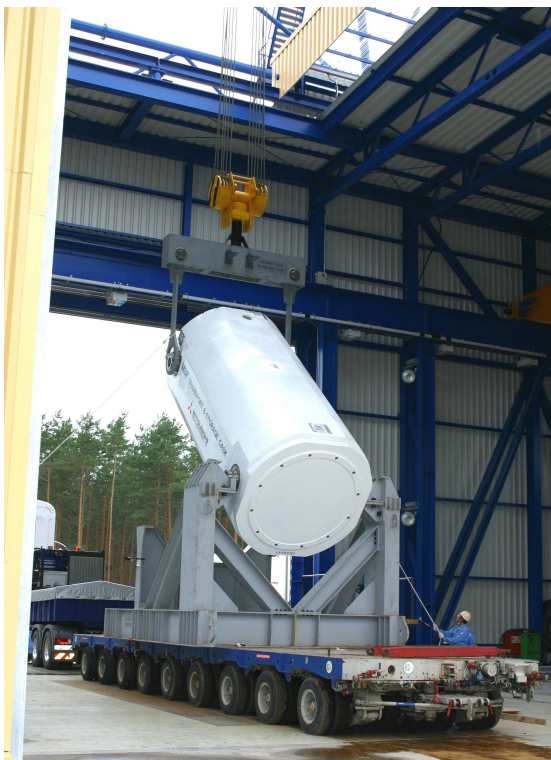
Fig. 3. Preparation of full-scale spent fuel casks for 9 meter drop testing at the BAM drop test facility.
