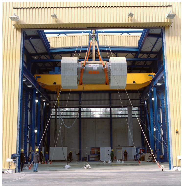
Fig. 3. Preparation of full-scale spent fuel casks for 9 meter drop testing at the BAM drop test facility.
