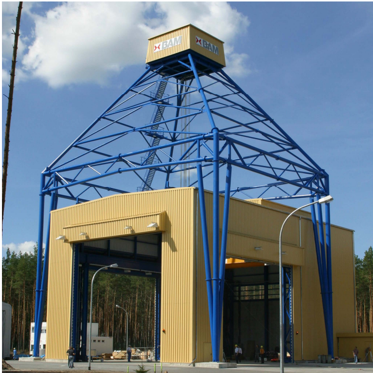
Fig. 2. BAM drop test facility in Horstwalde for big full-scale cask: Overall view and detaching device for test object's mass up to 200,000 kg.
