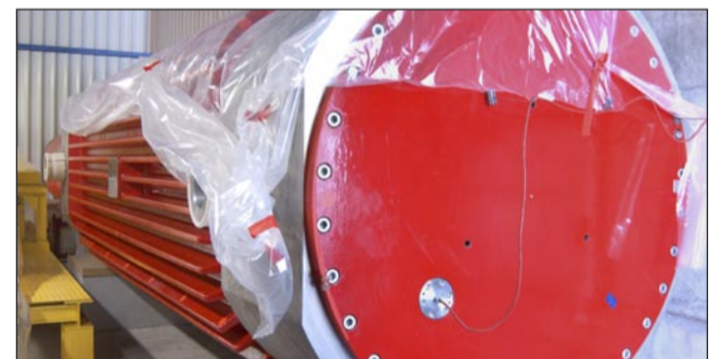
The CASTOR cask was stored at PSI from 1983 until mid-2004. It has been continuously monitored: passive leak-tightness control of the closure lids as well as the surface dose and temperature.
