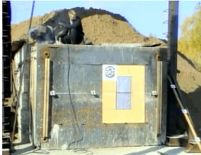
Fig.3. General view of the target designed to conduct impact tests on packages
