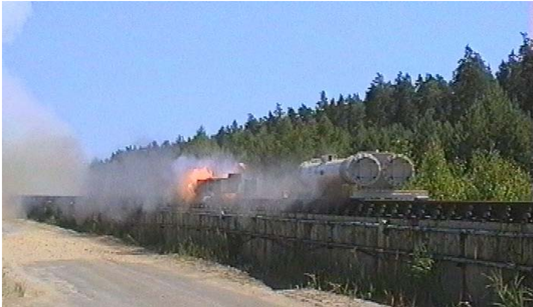
Fig.1. RFNC-VNIIEF horizontal rocket track used to test on shock impact of packages on a target with the velocity of not less than 90m/s
