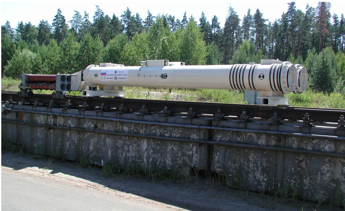
Fig.2. Rocket train containing TK-C5 package on rail guides of the horizontal rocket track
