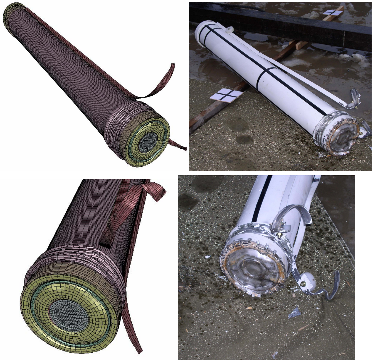
Fig.9. Comparison between the experiment and simulation of the impact of the TK-C7 package on the target with the velocity of 90 m/s
