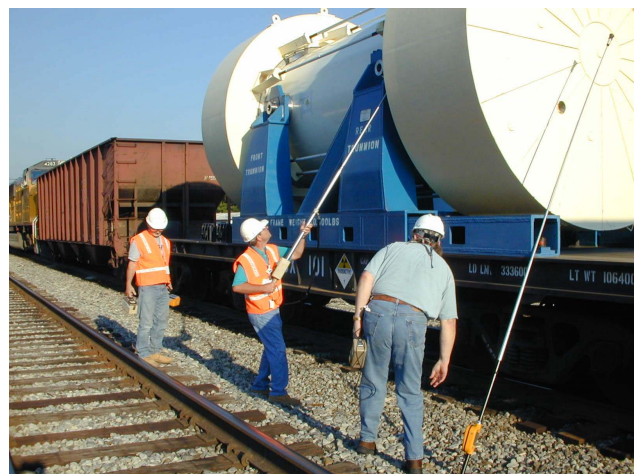
Figure 6. Photograph of en route radiological inspection of a railcar and cask.
