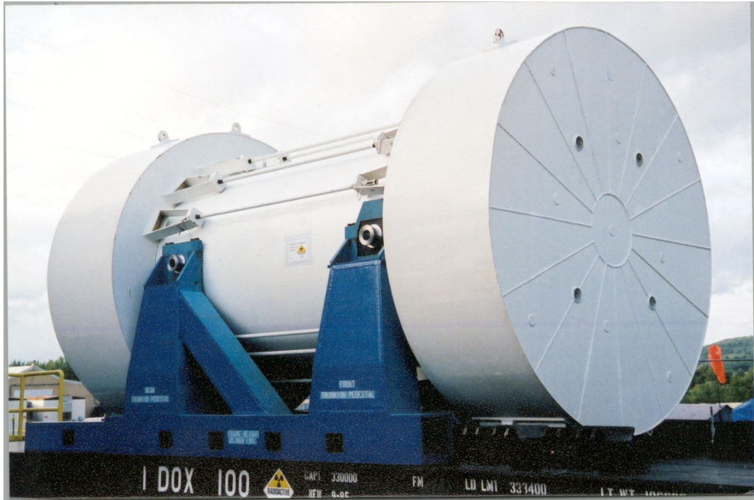
Figure 3. Photograph of a loaded West Valley cask with the impact limiters and tie rods installed.
