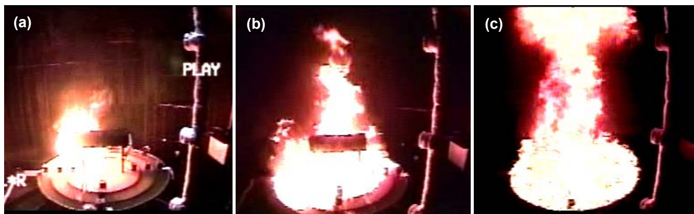
Figure 2. Controlled indoor fire (a) at the moment of ignition, (b) spreading over the pool, and (c) fully developed.
