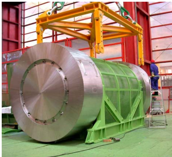
Photo 1 - NAC-STC Cask on the Transport Skid with Horizontal Lift Beam Above It
