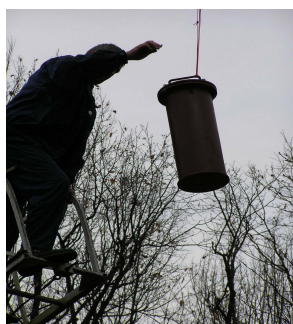
Figure 6 the type B (U) container subjected to the 1m free drop test.
