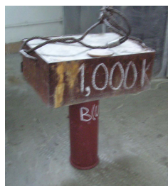
Figure 3 the type B (U) package subjected to the stacking test
