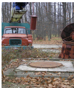
Figure 5 The 1.2 m free drop test for the Type B (U) package
