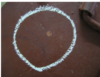
Figure no. 4 the type B (U) package after the penetration test
