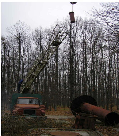
Figure 7 the type B (U) container during performing the 9 m free drop test
