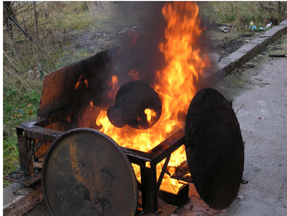
Figure 8 the type B (U) container during performing of the thermal test
