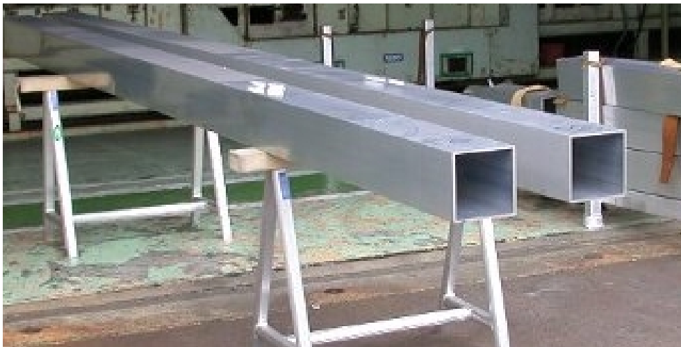
Figure 6 Tubes Made of Aluminum Alloy containing Neutron Absorbing Material
