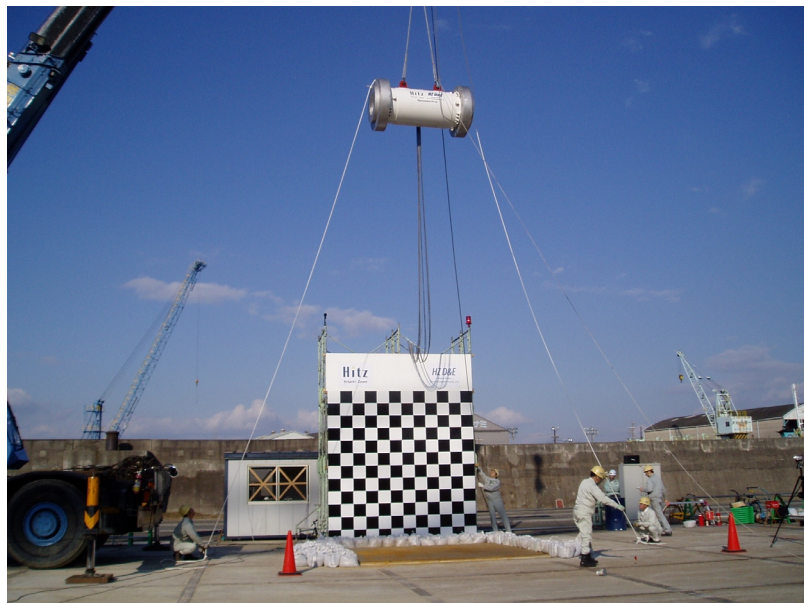
Figure 4 Scale Model 9m Drop Test
