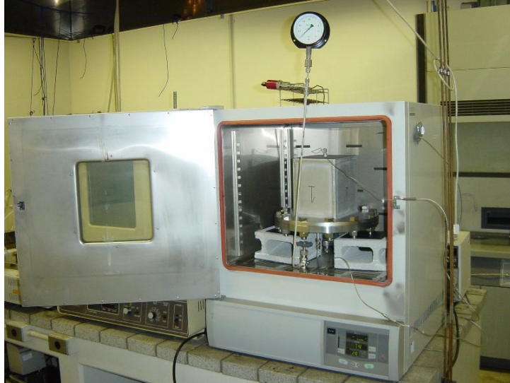
Figure 5 Resin Heat Degradation Test
