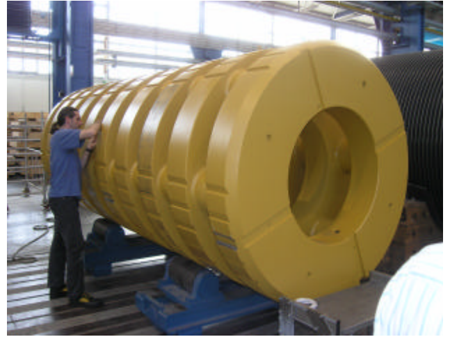
Fig. 3 CONSTOR® V/TC dummy basket
