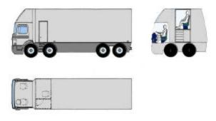
The above mentioned concept is based on a motor truck with a removable container, which also contains the TRP's compartment. The total weight, including 14,000 kg payload, was estimated to be 39,000 kg. Due to this, the concept was dropped out, because in Germany, this type of vehicle only is authorised up to a maximum total weight of 32,000 kg without heavy load authorisation
