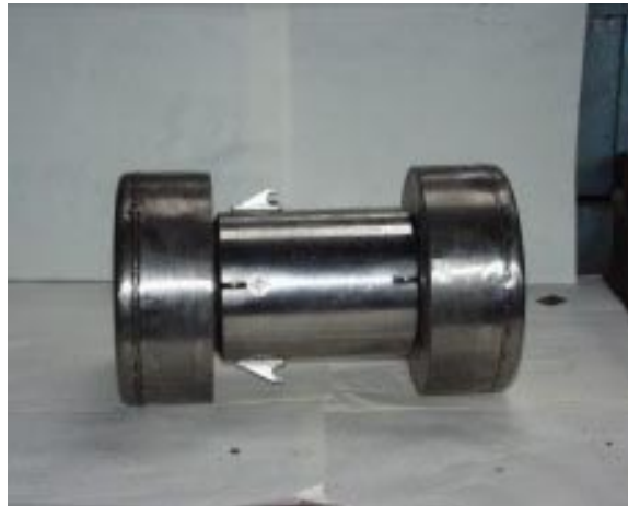
Figure 1 \frac{1}{4} Scale model type B container
