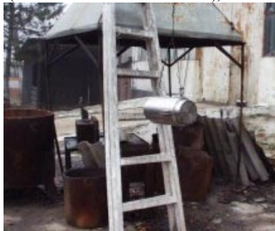
Figure 3. The 1/4 scale model prototype subjected to the 1.2 m free drop test (on the generator)
