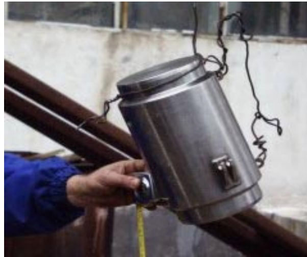
Figure 4. The \frac{1}{4} scale model prototype subjected to the 1.2 m free drop test ( on the lid with a 25° inclination )
