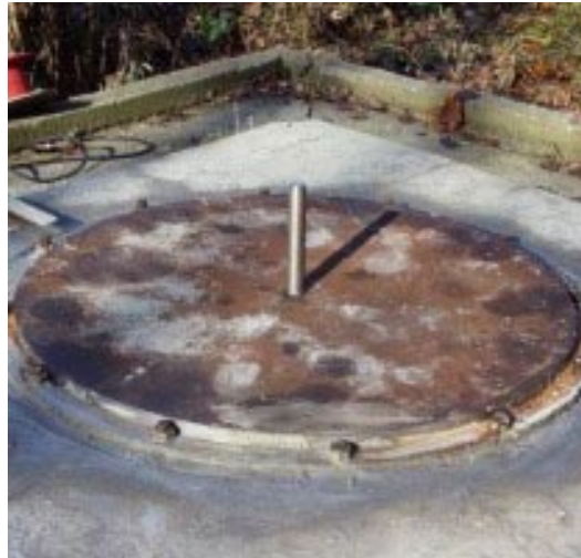
Figure 2 The target having the rigidly mounted 150 mm diameter mild steel bar mounted.
