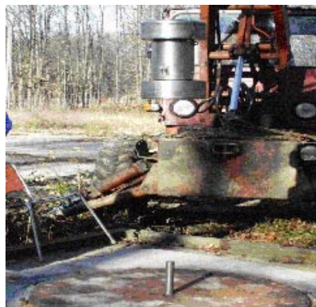
Figure 5. The \frac{1}{4} scale model prototype subjected to the 1 m free drop test (on the lid)
