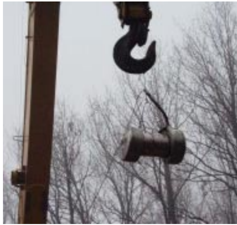
Figure 8. The package subjected to the 9m free drop test on the generator
