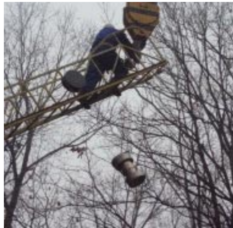
Figure 9. The package subjected to the 9 m free drop test with 25° inclination
