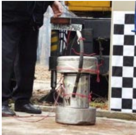
Figure 7. The container prepared before 9 m free drop testing (with shock absorbers mounted)
