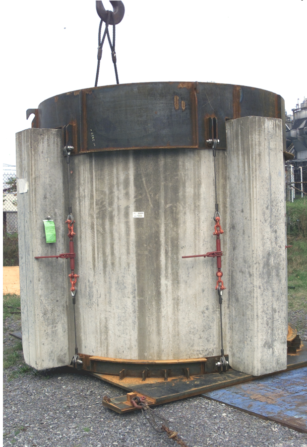
Fig. 1. Melton Valley Storage Tank package with the steel lid-retaining device in place.
