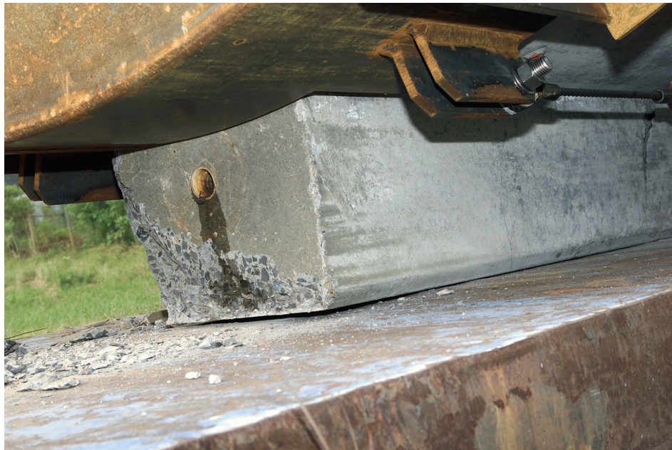
Fig. 3. The top steel cap of the lid-retaining device undamaged after the test.
