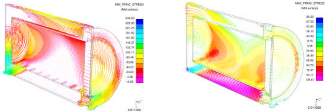
Figure 4, Side drop – Minimum and maximum principal stresses in the containment structure
