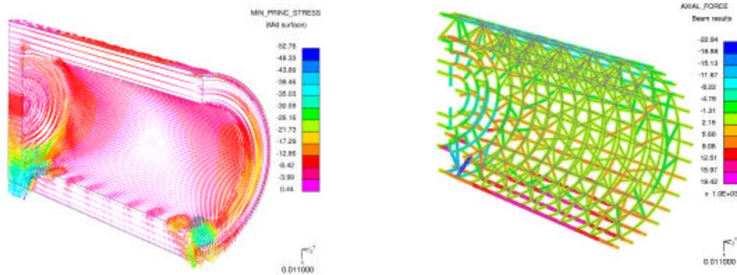
Figure 5, Side drop – Minimum principal stresses in the concrete and axial forces in the reinforcements
