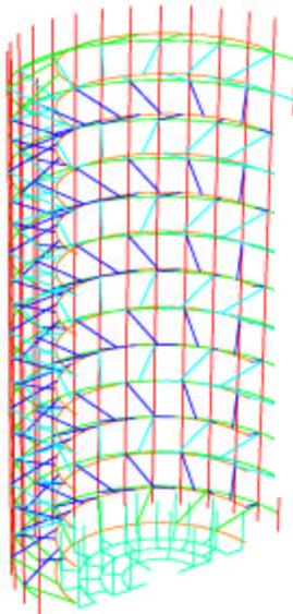
Figure 2, Model of reinforcement bars
