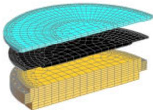
Figure 1, Model of cask body and lid – top half (steel structure only)
