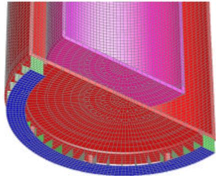
Figure 3, Model of lower half of cask body model (steel structure only)
