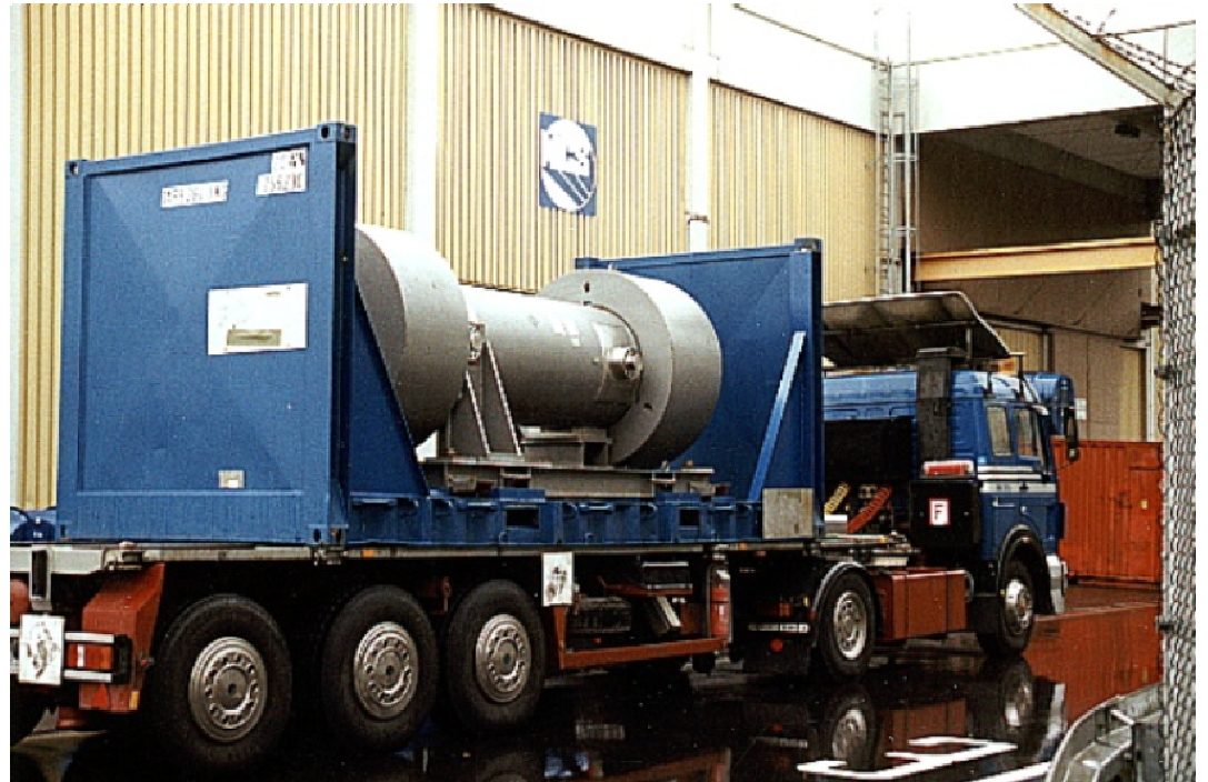
Transport of cask "TN 7-2" on 20ft. flat
