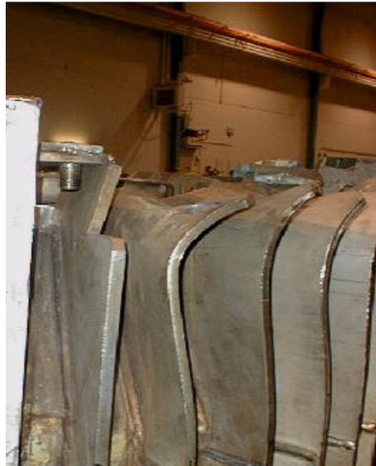
Figure 2. Typical Fin Deformation
