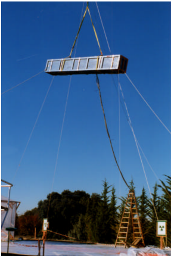
Fig. 8: RA-3D in position for 9 m slap down drop (f)
