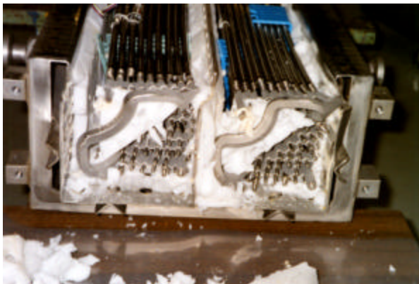
Fig. 6: deformation of the handles after test sequence no. 1
