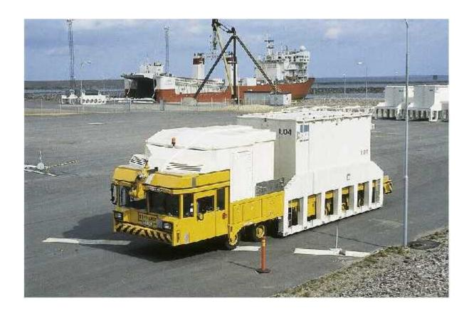
The ATB-8K will be transported from the Swedish Nuclear Power Plants by road on the specific trailer shown below to the plant harbor where it will be loaded on the M/S Sigyn. Then it will be transported by sea to the Swedish final storage facility, SFR, located in Forsmark where it will be unloaded.
