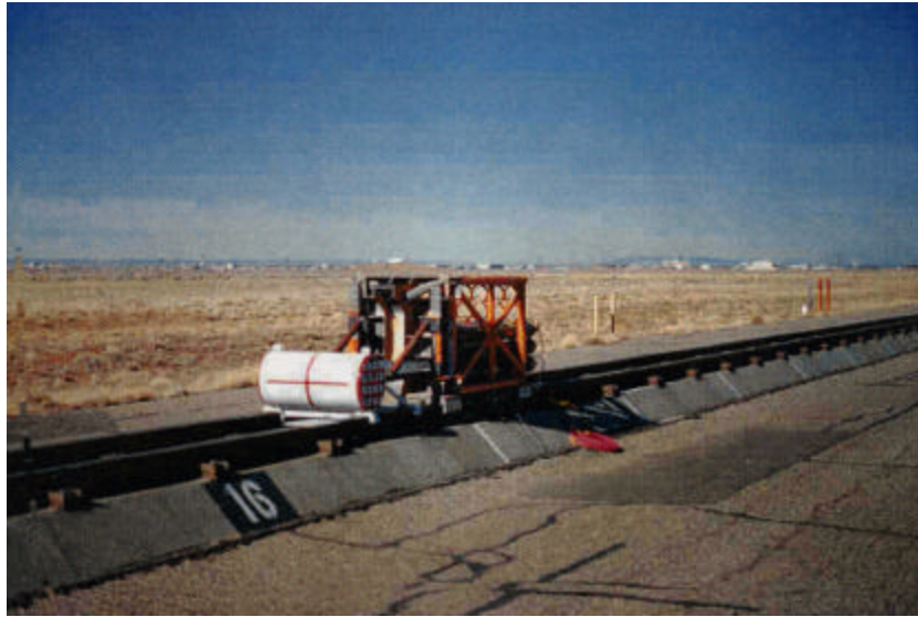
Figure 7. PMATP-SO1 and Pusher Sled Prior to Test
