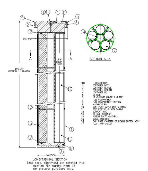
Figure 2 Arrangement of Oak Ridge Container in the TN-FSV Cask
