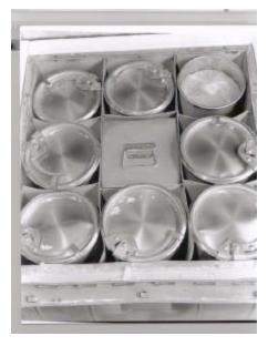
The main problems were with the steel lattice. As there was no restraint for the circular pails apart from this lattice they were relatively free to move. This caused distortion of the dividers which allowed the lid closures to contact each other causing damage. In addition the steel lattice distorted due to the impacts (see fig left).
