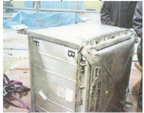
of a non-containment weld between angles and flange. There was further bowing of the package faces.
