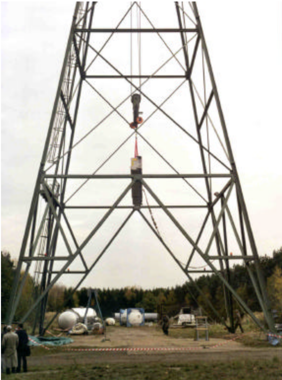
Fig. 3 9 m Drop Test with the ANF-18 Container
