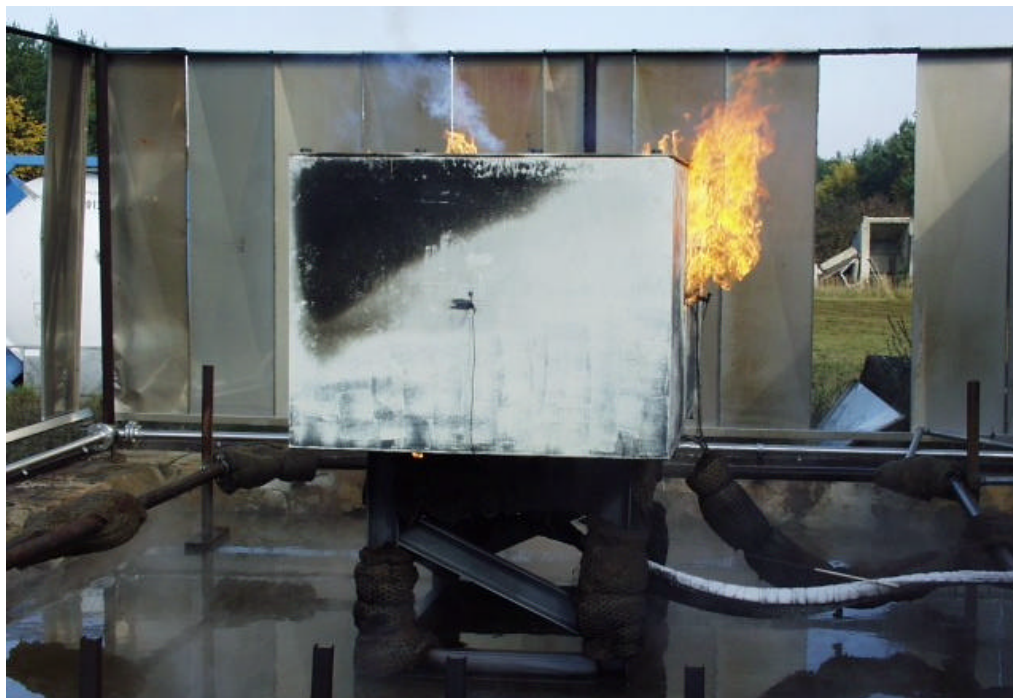
Fig. 6 Test Segment of the Outer Protective Packaging After the Thermal Test
