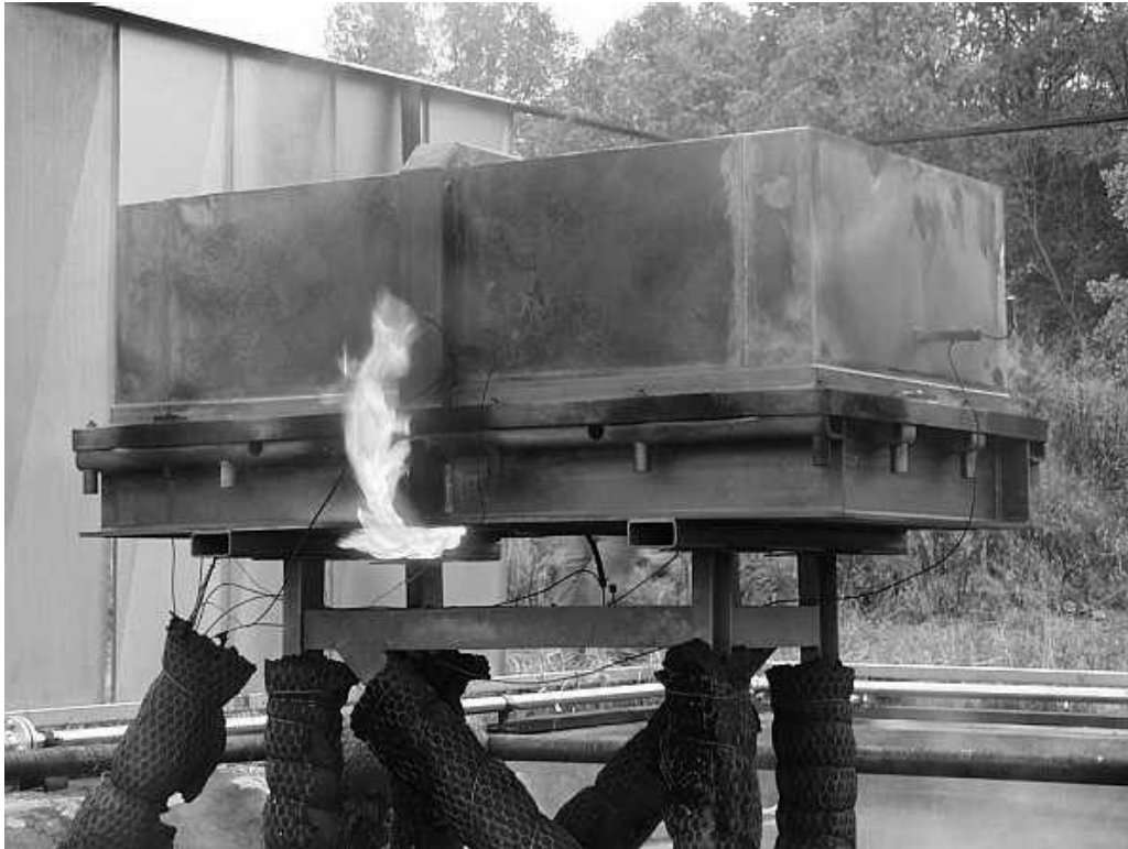
Fig. 5 ANF-18 Test Segment After Fire Test
