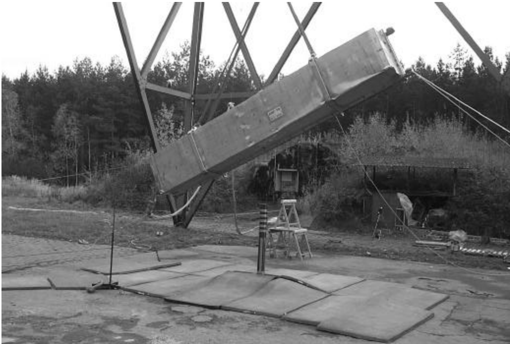
Fig. 4 ANF-18 Bar Drop Test from a Height of 1.1 m
